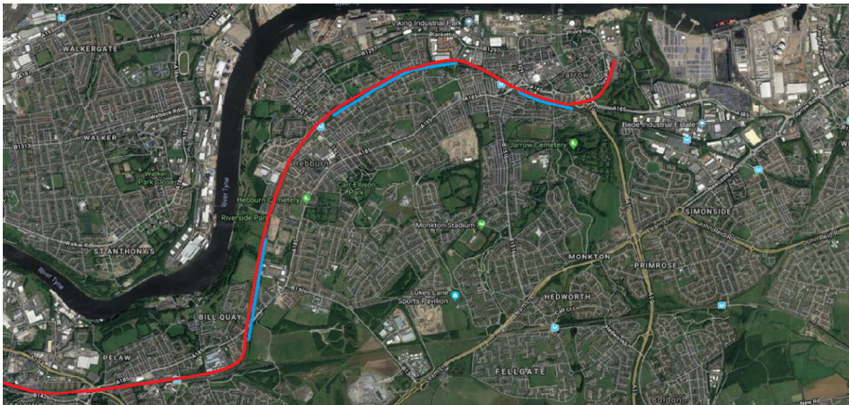
Figure 11: Pelaw to Bede - Network Rail line shown Red, single-track Metro sections in Blue
